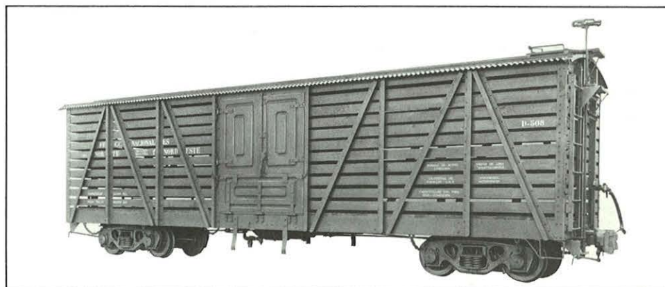
Composite cattle cars for Colombia; spring-plankless bogies with Timken roller bearings. Capacity: 25 metric tons. Track Gauge: 3'-0".
