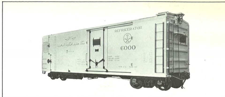
Refrigerator cars for Saudi Arabia equipped with diesel-powered refrigeration and Gregg-Barber stabilized trucks. Capacity: 40 tons. Track Gauge: 4'-8½".
