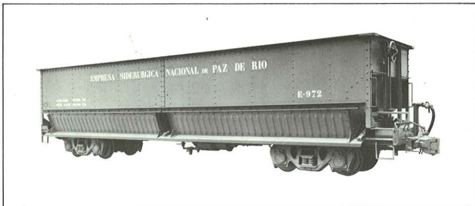
Gable-bottom coal cars for Colombia; self-aligning bogies with Timken bearings. Capacity: 50 metric tons. Track Gauge: 3'-0".
