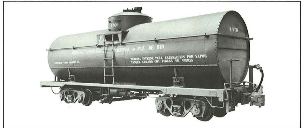
Insulated tank cars with internal heating coils; cast-steel bogies with Timken bearings. Capacity: 6,000 gallons. Track Gauge: 3'-0".
