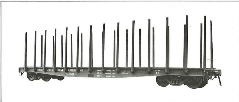
Flat cars with removable stakes for oil well casings; Gregg-Barber stabilized bogies with Unit brake beams and Timken AP bearings. Capacity: 50 tons. Track Gauge: 4'-8 1/2". Platform Size: 46'-9" x 9'-4".
