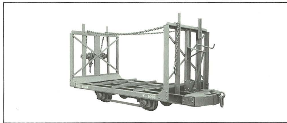
Cane cars for Uganda with 12" cast steel wheels, roller bearings and screw hand brake; car equipped with hold-down chains and windlass. Capacity: 4 tons. Track Gauge: 610 mm (24").
