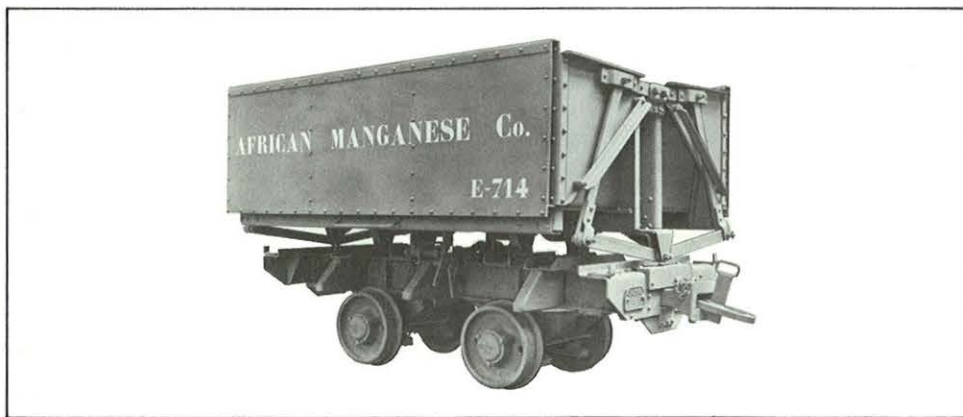
Box dump ore cars for Ghana; 20" wheels with self-contained roller bearings. Capacity: 5 cubic yards. Track Gauge: 2'-6".
