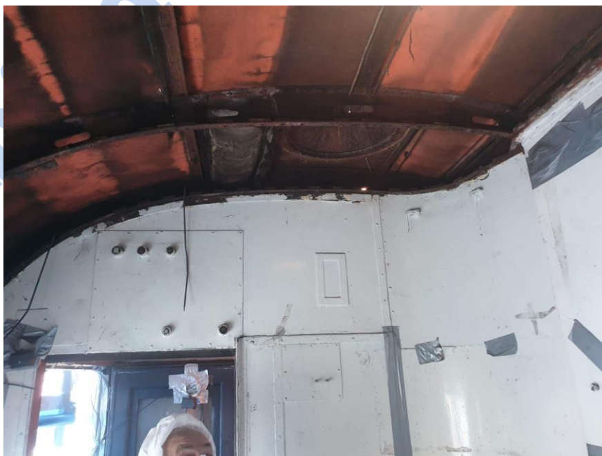
WR 2975 – Cuisine roof after asbestos removal – Nene Valley Railway 2019
