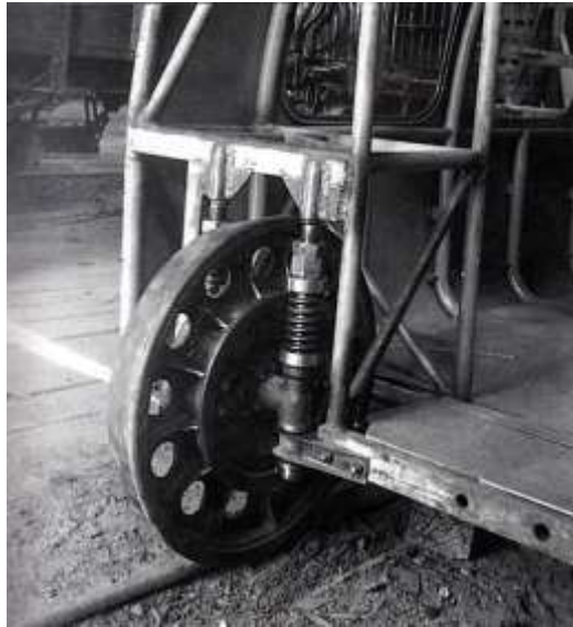
Talgo01_04 Valladolid 1944. Detail of rudimentary intermediate car suspension of Talgo I
