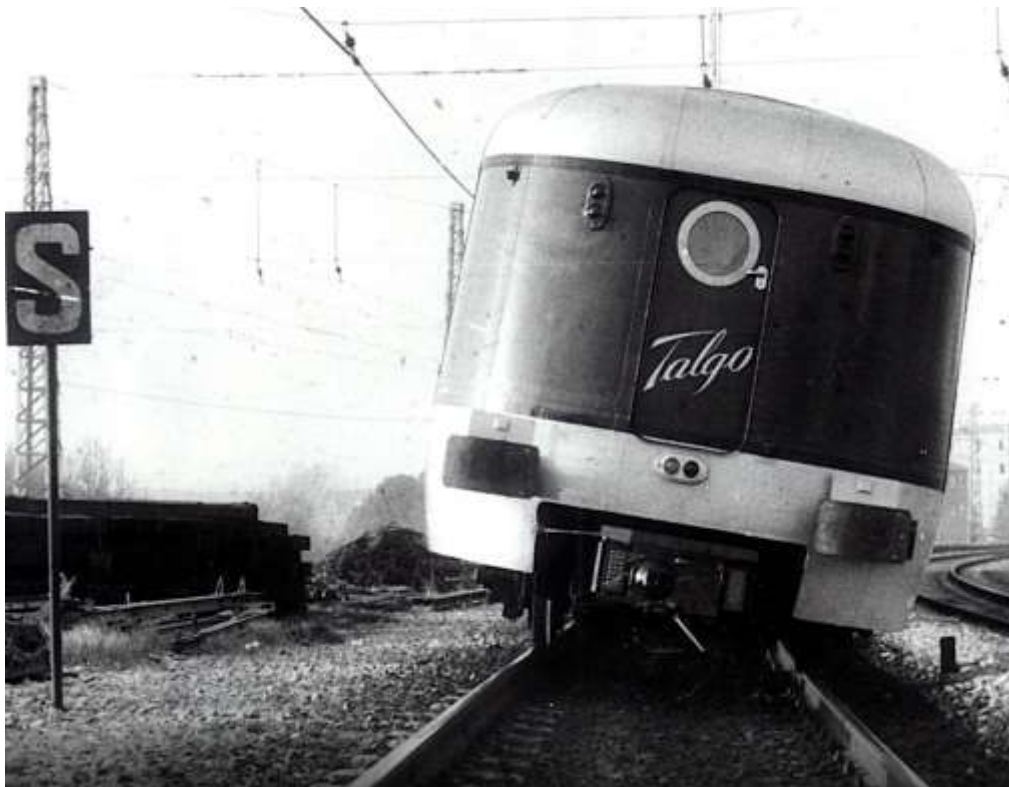
Talgo01_15 Madrid 1977. Prototype Pendular rounding curve, showing a potential coupling angle problem at rear.
