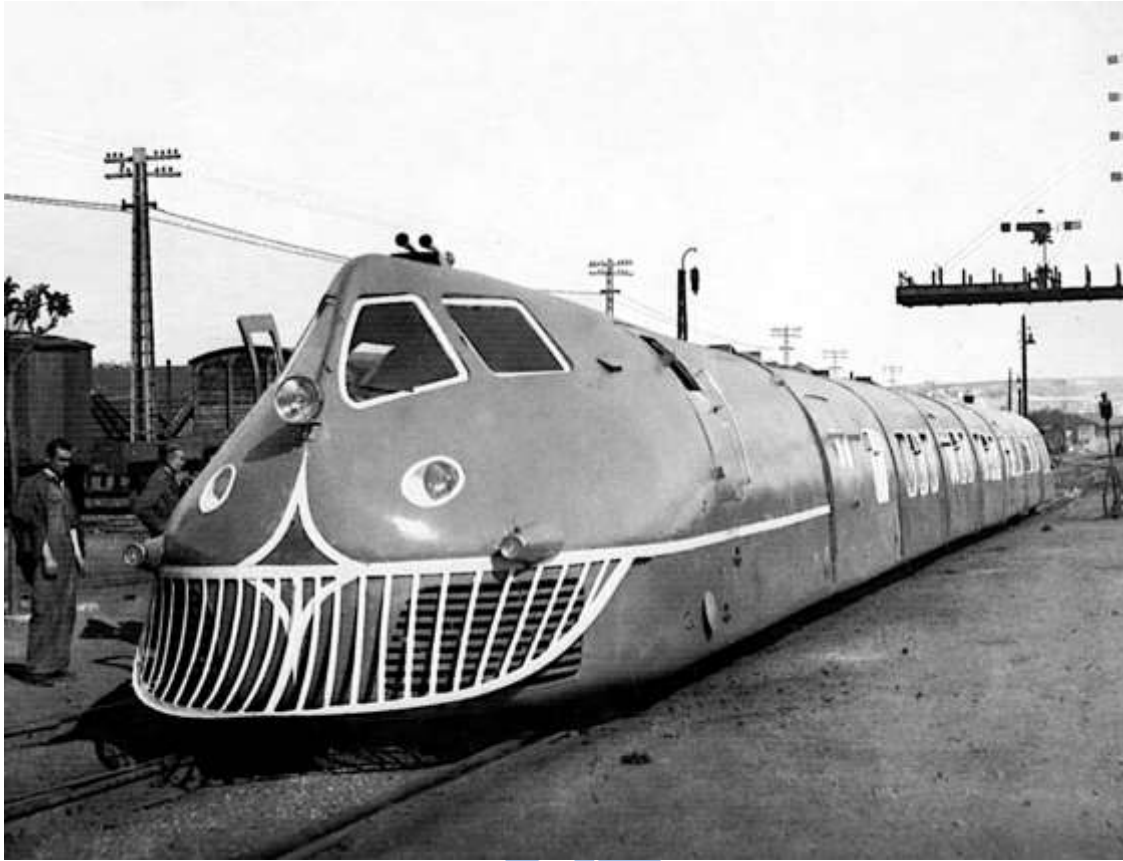
Talgo01_02 Aranjuez 1944. Talgo I prototype during testing between Madrid and Aranjuez with the Ganz railcar chassis hidden by 'streamlining'.
