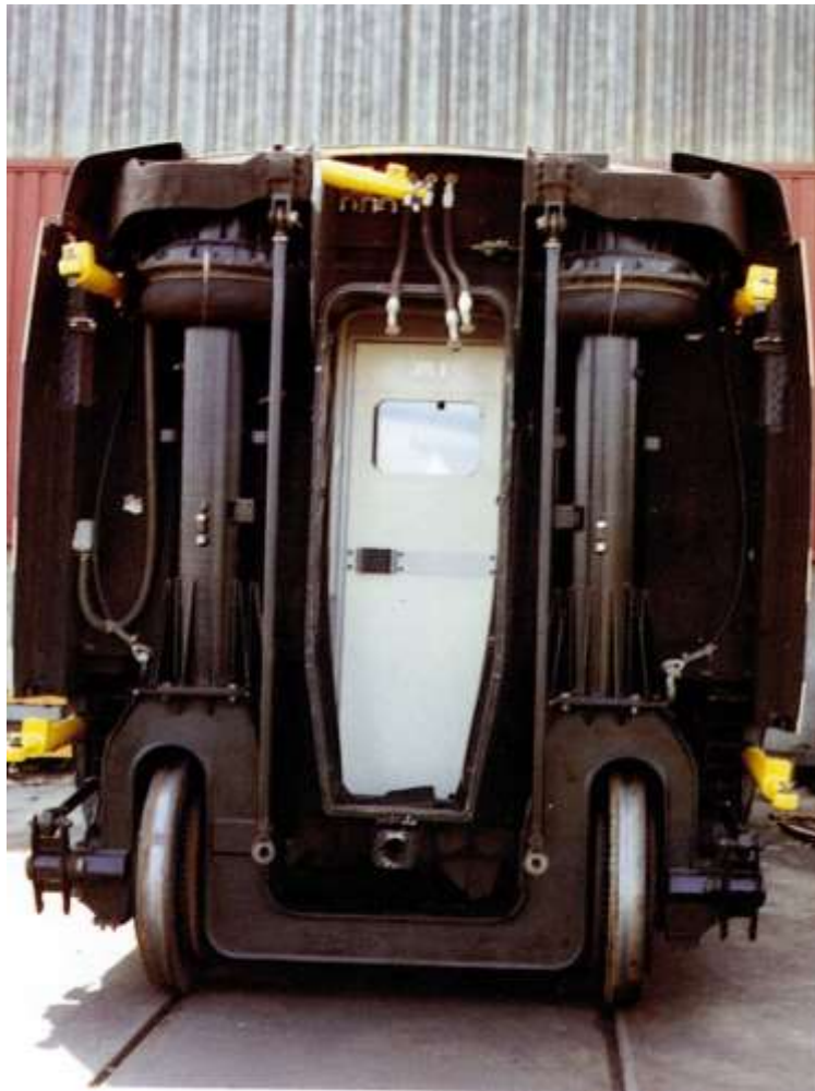
Talgo01_17 Typical Talgo Pendular suspension arrangement (Series V) note disc brakes.
