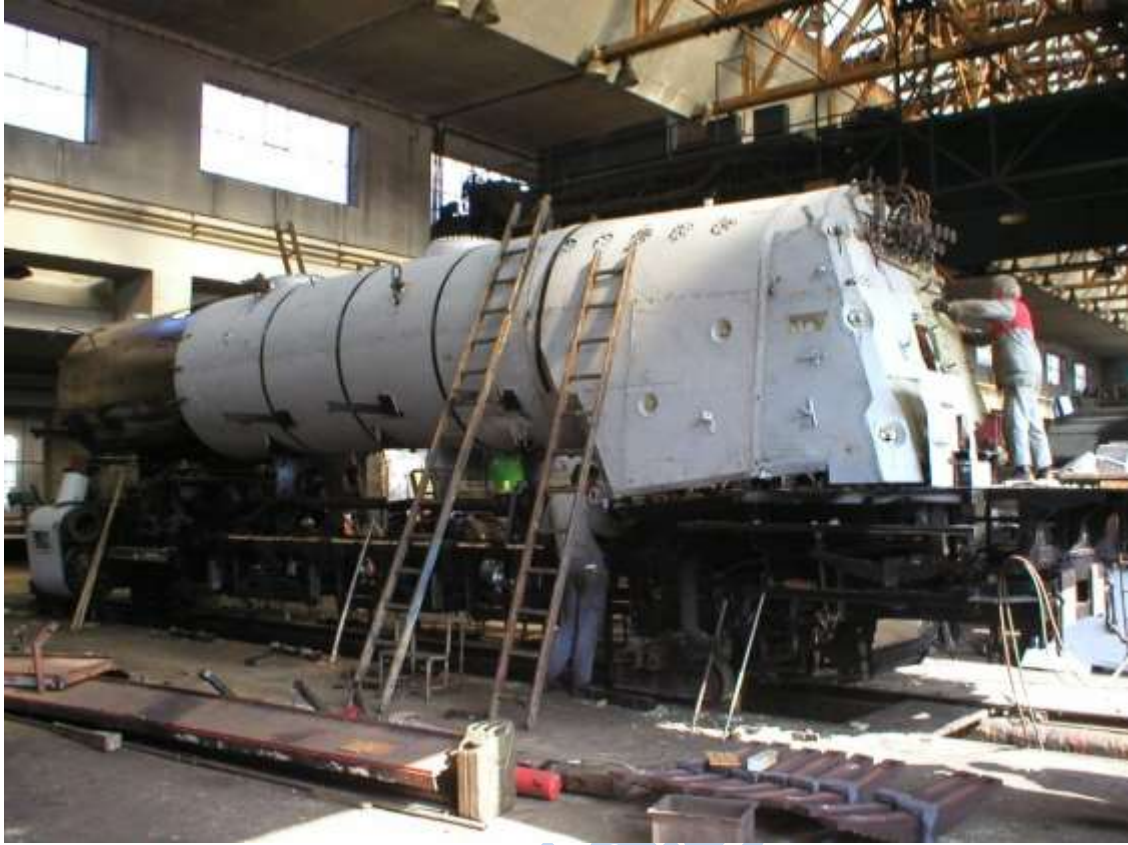
04_CK_2004.jpg here: Škoda-built ČSD 2-D-1 loco 475.179 undergoing overhaul at ŽOS České Velenice in 2004 (SŽND).
