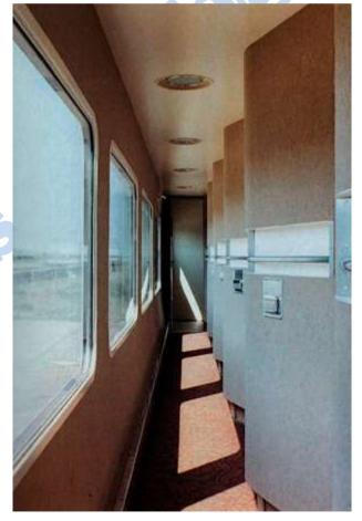
The corridor of a Talgo-III RD Camas sleeping car showing the staggered formation of the compartments (Talgo).
