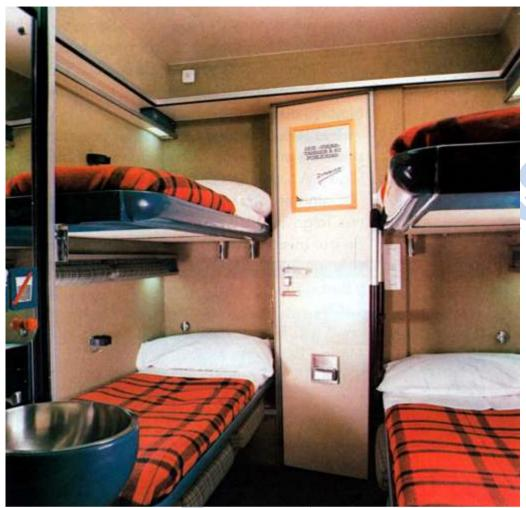
The compartment of a staggered Talgo-IV 2<sup>nd</sup> class T4 sleeping car (Talgo).
