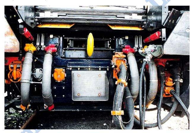
A front-end of view of a Nightstar Type 1 car connection (H. Scherpenhuizen).
