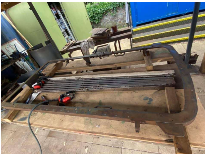
Gangway connection cover ready for painting.
