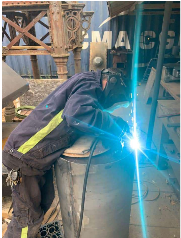
The inner cylinder with its tubes for increasing the surface area ready to be welded (left). Joel welding the outer cylinder of the heater (right).
