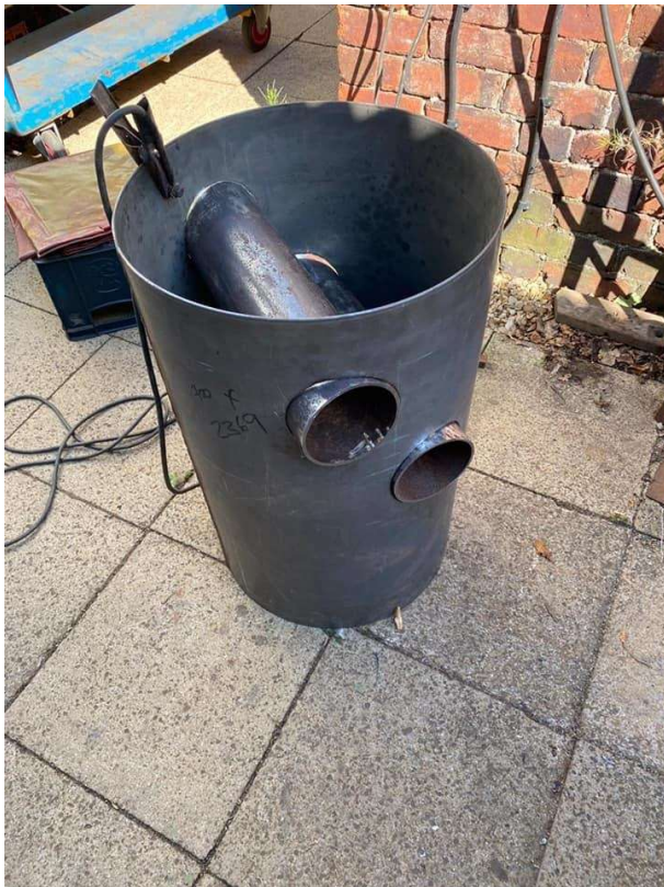
The inner cylinder with its tubes for increasing the surface area ready to be welded (left). Joel welding the outer cylinder of the heater (right).
