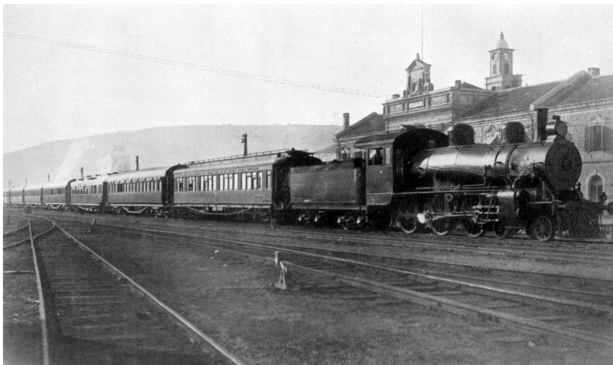
Cairo Express at Haifa East in 1934: Behind the locomotive the WL type R18 from MAN or van der Zypen & Charlier (from numbers 1774, 1777, 1778, 1780, 2072 and 2168), in third place the WR from Ringhoffer (from numbers 2302, 2346 and 2351). The course WL from Jerusalem is not present in Haifa. (Photo: Cotterel archive)
