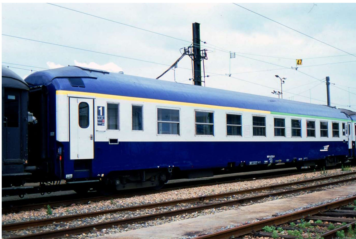
French (SNCF) UIC-Y Couchette car A4c4B5c5 44-70 341 with first and second class compartments in Paris Massena on 3 July 1996, Coll. DF.
