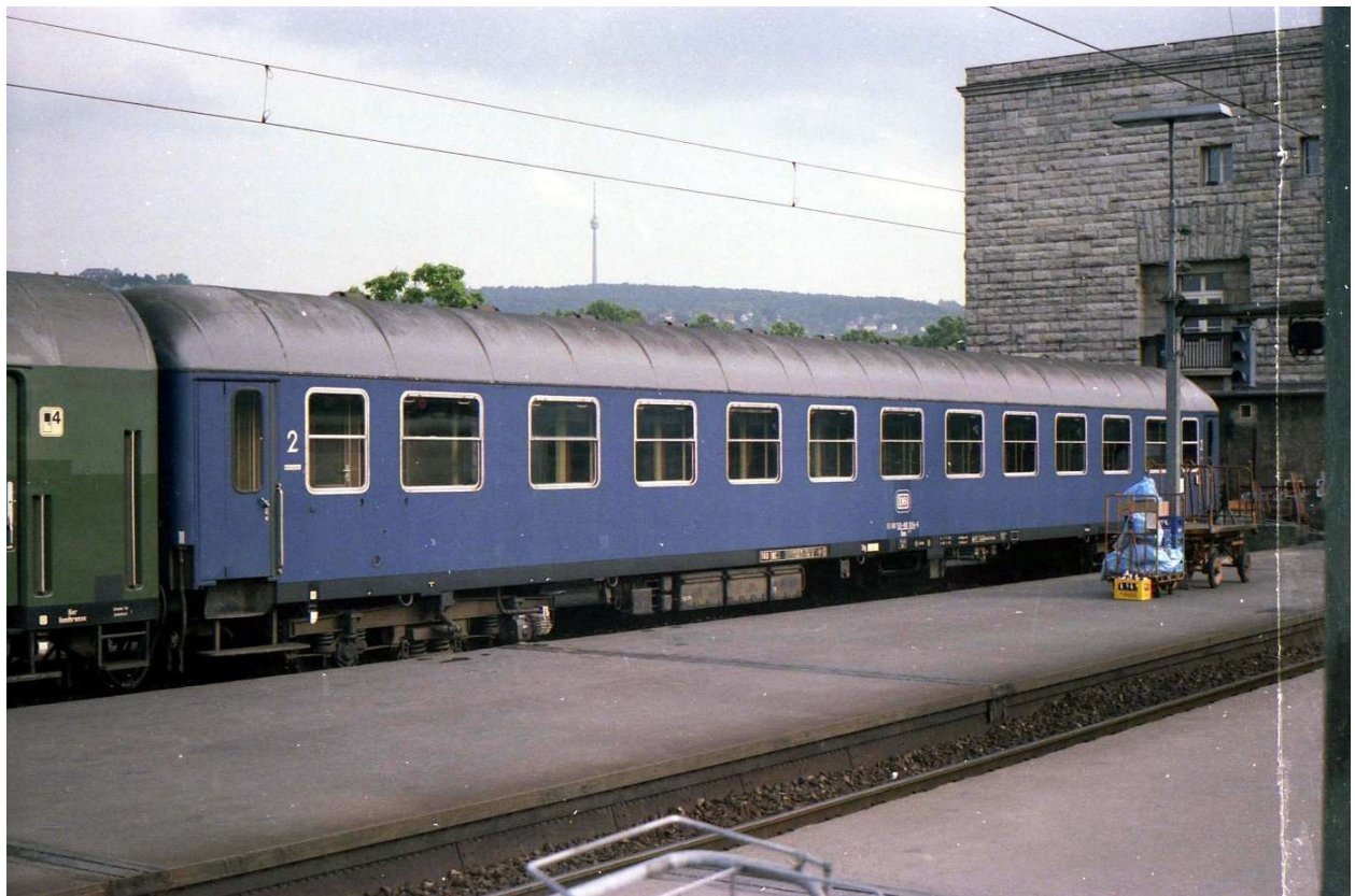
Bcm 243 DB UIC-X Couchette car no. 50-80 094 in Stuttgart Hbf in 1984, coll. DF.
