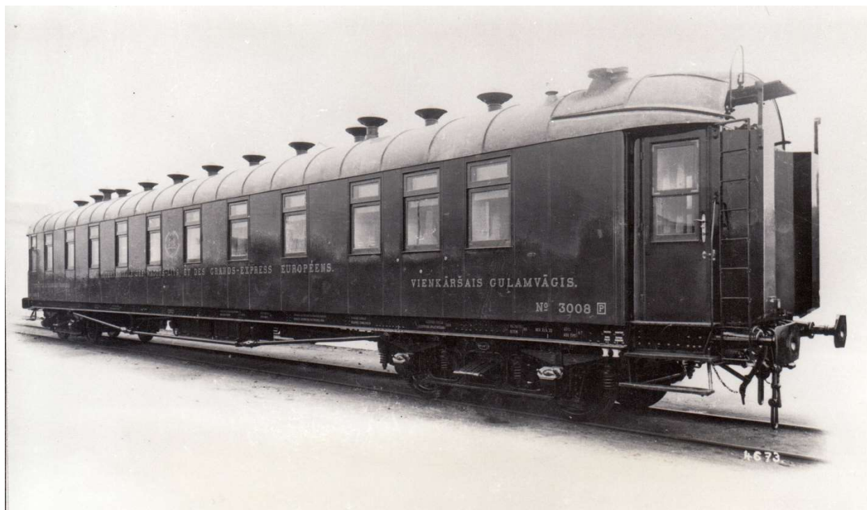
CIWL No. 3008 type III sleeping car – built by Ringhoffer wagon works in Prague-Smichov in 1925. Work's photograph, Toms Altbergs collection.
