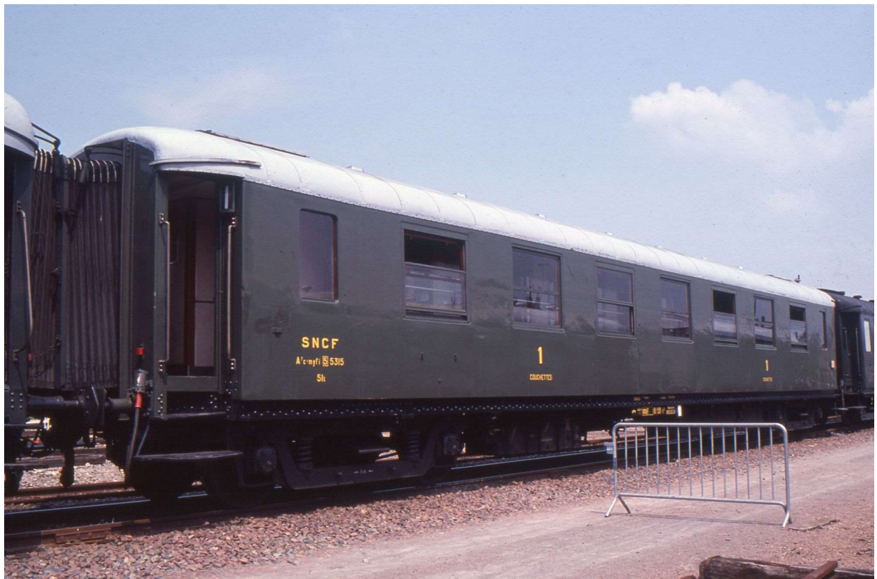
Couchette coaches - in pre-war times almost first class and on the same level as the CIWL with bedding and washing facilities, in post-war times the means of transport of choice for night journeys by trampers and families. The picture shows a first class couchette car ex PLM A7c7 of the SNCF, now preserved by AJECTA.
