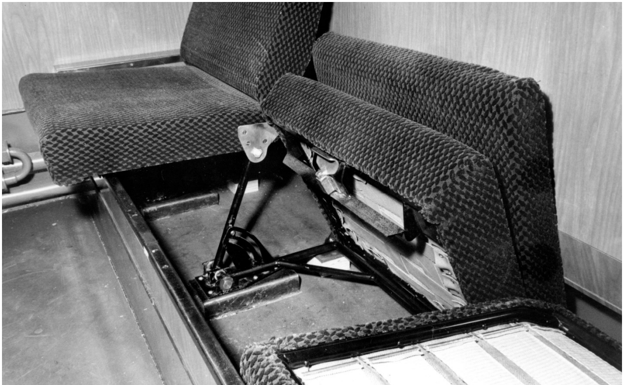
The folding mechanism from day to night for readjusting the seat.
