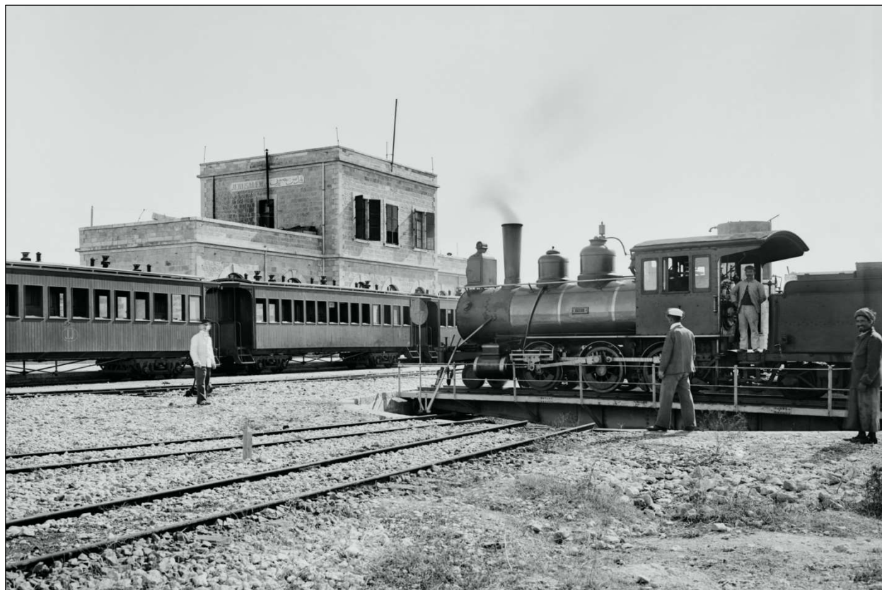
A Baldwin 2-6-0 on the Jerusalem turntable about 1900 - Collection: Historical Museum of Tel Aviv 14
